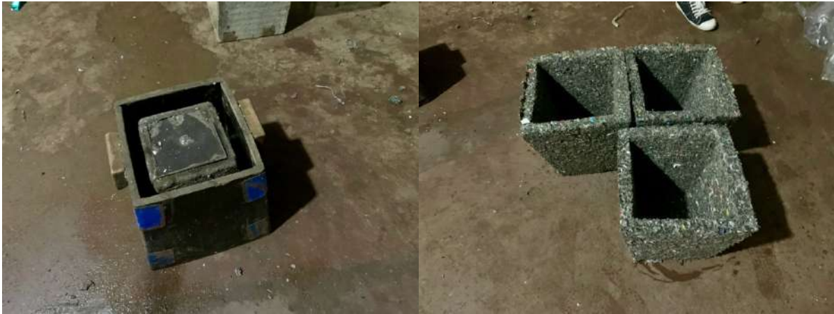
Figure 9: Downcycling mold (left) and downcycled flower pots (right) (Source: Photos taken during field visit)
