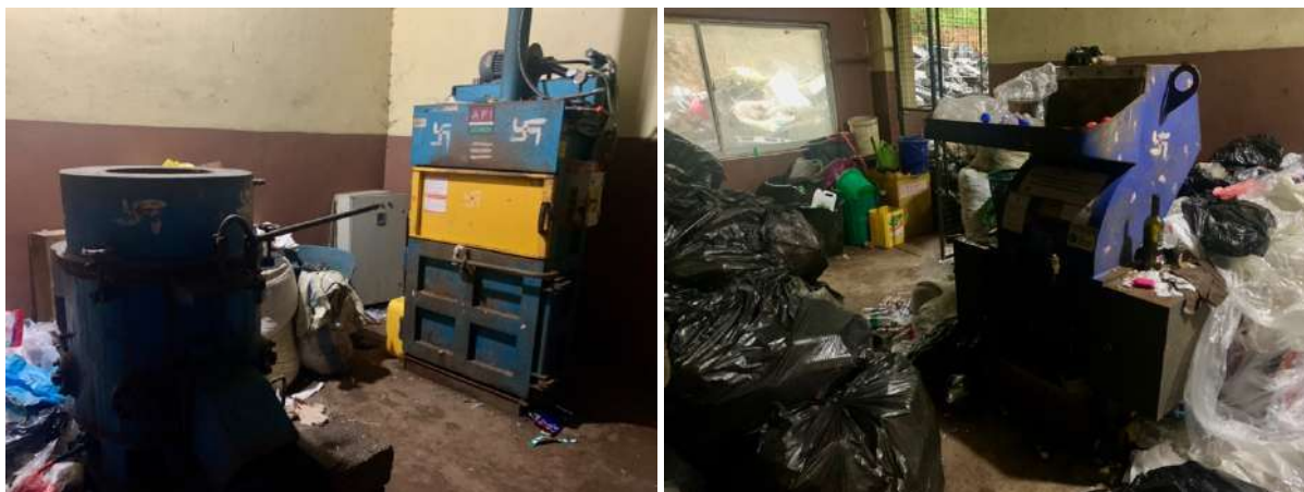
Figure 8: Plastic press and downcycling machine (left) and shredder (right) (Source: Photos taken during field visit)
